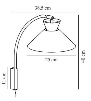
Voltage (V): 220-240 Volt IP degree: IP20 Maximum bulb wattage (W): 40 Class (Class 1, Class 2, Class 3): Class 2 (Double isolated) Socket type: E27 Switch placement: On the cable Parallel connection: False
