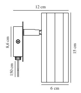
Voltage (V): 220-240 Volt IP degree: IP20 Maximum bulb wattage (W): 15W Class (Class 1, Class 2, Class 3): Class 2 (Double isolated) Socket type: GU10 Switch placement: On the fixture Parallel connection: False
