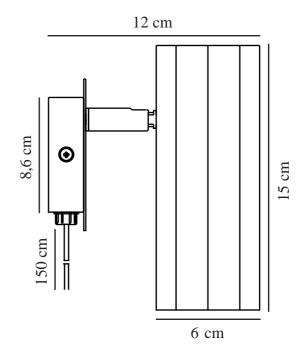
Voltage (V): 220-240 Volt IP degree: IP20
