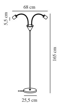
Voltage (V): 220-240 Volt IP degree: IP20 Maximum bulb wattage (W): 7W Class (Class 1, Class 2, Class 3): Class 2 (Double isolated) Socket type: GU10 Switch placement: On the cable Parallel connection: False
