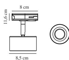
Voltage (V): 220-240 Volt IP degree: IP20 Class (Class 1, Class 2, Class 3): Class 2 (Double isolated) Socket type: LED – Nonreplaceable light source Parallel connection: False
