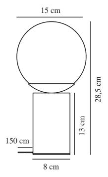
Voltage (V): 220-240 Volt IP degree: IP20 Maximum bulb wattage (W): 25 Class (Class 1, Class 2, Class 3): Class 2 (Double isolated) Socket type: E14 Switch placement: On the cable Parallel connection: False
