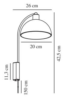
Voltage (V): 220-240 Volt IP degree: IP20
