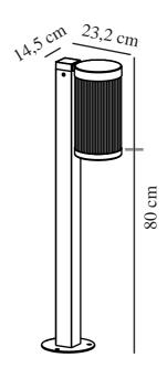
Voltage (V): 220-240 Volt IP degree: IP54
