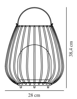
IP degree: IP54 Class (Class 1, Class 2, Class 3): Class 3 (12V) Socket type: LED – Nonreplaceable light source Switch placement: On the table/ground base
