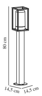
Voltage (V): 220-240 Volt IP degree: IP44 Maximum bulb wattage (W): 15W Class (Class 1, Class 2, Class 3): Class 1 (Earth contact) Socket type: E27 Parallel connection: True
