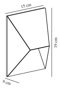
Voltage (V): 220-240 Volt IP degree: IP54 Maximum bulb wattage (W): 25 Class (Class 1, Class 2, Class 3): Class 1 (Earth contact) Socket type: GU10 Parallel connection: True
