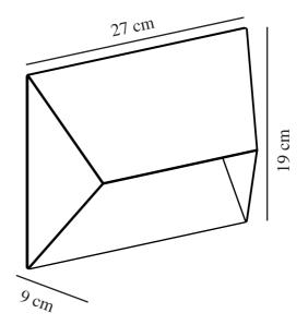
Voltage (V): 220-240 Volt IP degree: IP54 Maximum bulb wattage (W): 25 Class (Class 1, Class 2, Class 3): Class 1 (Earth contact) Socket type: GU10 Parallel connection: True
