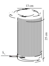
Voltage (V): 220-240 Volt IP degree: IP54 Maximum bulb wattage (W): 25W Class (Class 1, Class 2, Class 3): Class 2 (Double isolated) Socket type: E27 Switch placement: On the cable Parallel connection: False
