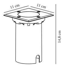
Voltage (V): 220-240 Volt IP degree: IP67 Maximum bulb wattage (W): 15 Class (Class 1, Class 2, Class 3): Class 1 (Earth contact) Socket type: GU10 Parallel connection: True
