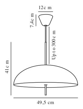
Voltage (V): 220-240 Volt IP degree: IP20 Maximum bulb wattage (W): 60 Class (Class 1, Class 2, Class 3): Class 2 (Double isolated) Socket type: E27 Parallel connection: False
