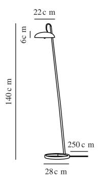
IP degree: IP20 Maximum bulb wattage (W): 3 Class (Class 1, Class 2, Class 3): Class 2 (Double isolated)
