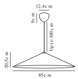
Voltage (V): 220-240 Volt IP degree: IP20 Maximum bulb wattage (W): 25 Class (Class 1, Class 2, Class 3): Class 2 (Double isolated) Socket type: E27
