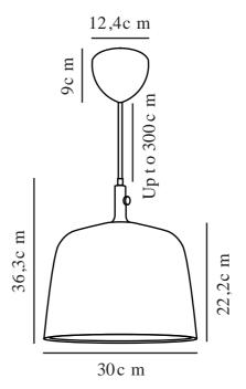
Voltage (V): 220-240 Volt IP degree: IP20 Maximum bulb wattage (W): 60W Class (Class 1, Class 2, Class 3): Class 2 (Double isolated) Socket type: E27
