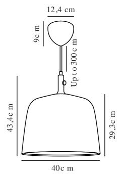
Voltage (V): 220-240 Volt IP degree: IP20 Maximum bulb wattage (W): 60W Class (Class 1, Class 2, Class 3): Class 2 (Double isolated) Socket type: E27
