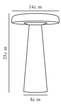
Voltage (V): 5 Volt IP degree: IP54 Class (Class 1, Class 2, Class 3): Class 3 (12V) Socket type: LED – Nonreplaceable light source Switch placement: Under the table/ground base Parallel connection: False
