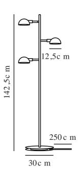
Voltage (V): 220-240 Volt IP degree: IP20 Maximum bulb wattage (W): 8 Class (Class 1, Class 2, Class 3): Class 2 (Double isolated) Socket type: E14 Switch placement: On the fixture
