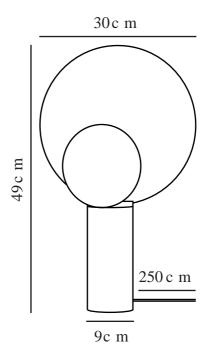
Voltage (V): 220-240 Volt IP degree: IP20 Maximum bulb wattage (W): 40 Class (Class 1, Class 2, Class 3): Class 2 (Double isolated) Socket type: GU10 Switch placement: On the cable
