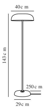
Voltage (V): 220-240 Volt IP degree: IP20
