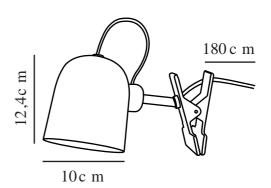
Voltage (V): 220-240 Volt IP degree: IP20 Maximum bulb wattage (W): 15 Class (Class 1, Class 2, Class 3): Class 2 (Double isolated) Socket type: GU10 Switch placement: On the cable
