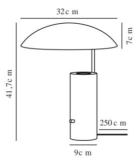
Voltage (V): 220-240 Volt IP degree: IP20 Maximum bulb wattage (W): 15 Class (Class 1, Class 2, Class 3): Class 2 (Double isolated) Socket type: GU10 Switch placement: On the
