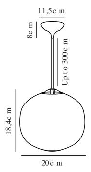
Voltage (V): 220-240 Volt IP degree: IP20 Maximum bulb wattage (W): 40 Class (Class 1, Class 2, Class 3): Class 2 (Double isolated) Socket type: E27
