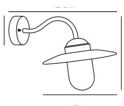
Voltage (V): 230 Volt IP degree: IP54 Maximum bulb wattage (W): 60 Class (Class 1, Class 2, Class 3): Class 2 (Double isolated) Socket type: E27 Parallel connection: True
