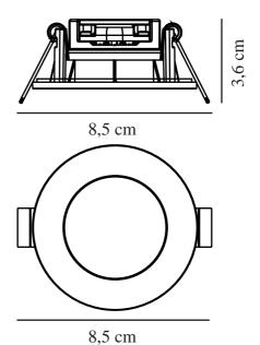
Voltage (V): 220-240 Volt IP degree: IP65 Class (Class 1, Class 2, Class 3): Class 2 (Double isolated) Socket type: LED - Nonreplaceable light source Dimmerable: False Parallel connection: True
