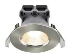
Voltage (V): 220-240 Volt IP degree: IP65 Class (Class 1, Class 2, Class 3): Class 2 (Double isolated) Socket type: LED Module Dimmerable: True Parallel connection: True
