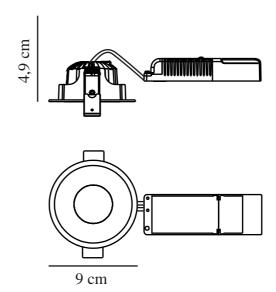
Voltage (V): 220-240 Volt IP degree: IP44 Class (Class 1, Class 2, Class 3): Class 2 (Double isolated) Socket type: LED – Nonreplaceable light source Parallel connection: True
