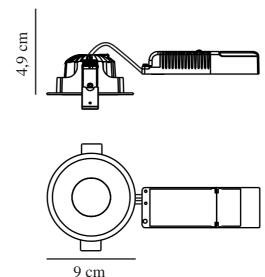
Tension (V): 220-240 Volt Protection IP: IP44 Classe (Classe 1, Classe 2, Classe 3): Classe 2 (Double isolation)
