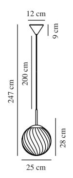
Voltage (V): 220-240 Volt IP degree: IP20 Maximum bulb wattage (W): 40W Class (Class 1, Class 2, Class 3): Class 2 (Double isolated) Socket type: E27 Parallel connection: False
