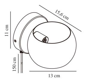
Voltage (V): 220-240 Volt IP degree: IP20 Maximum bulb wattage (W): 5W Class (Class 1, Class 2, Class 3): Class 2 (Double isolated) Socket type: G9 Switch placement: On the cable Parallel connection: False
