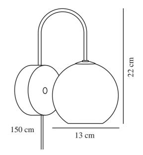
Voltage (V): 220-240 Volt IP degree: IP20 Maximum bulb wattage (W): 40W Class (Class 1, Class 2, Class 3): Class 2 (Double isolated) Socket type: E14 Switch placement: On the base Parallel connection: False
