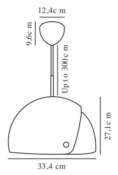
Voltage (V): 220-240 Volt IP degree: IP20 Maximum bulb wattage (W): 15W Class (Class 1, Class 2, Class 3): Class 2 (Double isolated) Socket type: E27 Parallel connection: False
