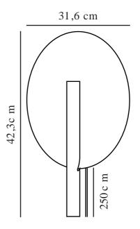
Voltage (V): 220-240 Volt IP degree: IP20 Maximum bulb wattage (W): 6W Class (Class 1, Class 2, Class 3): Class 2 (Double isolated) Socket type: G9 Switch placement: On the cable
