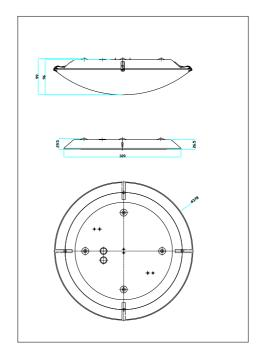
Voltage (V): 220-240 Volt IP degree: IP20 Maximum bulb wattage (W): 60W Class (Class 1, Class 2, Class 3): Class 1 (Earth contact) Socket type: E27 Parallel connection: True
