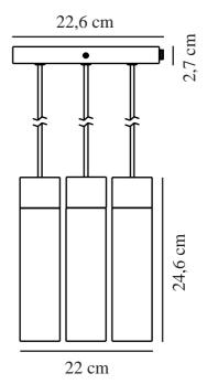
Voltage (V): 230 Volt IP degree: IP20 Maximum bulb wattage (W): 3x15W
