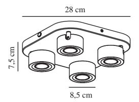
Voltage (V): 220-240 Volt IP degree: IP20
