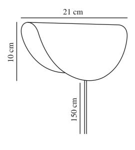
IP degree: IP20 Maximum bulb wattage (W): 25 Class (Class 1, Class 2, Class 3
