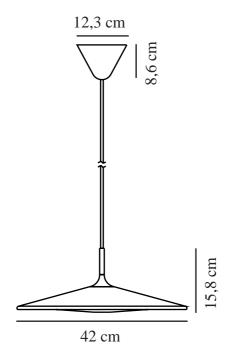
Tension (V): 220-240 Volt Protection IP: IP20 Classe (Classe 1, Classe 2, Classe 3): Classe 2 (Double isolation)
