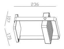
Voltage (V): 5 Volt IP degree: IP44 Class (Class 1, Class 2, Class 3): Class 3 (12V) Socket type: LED Module Switch placement: On the fixture Parallel connection: False
