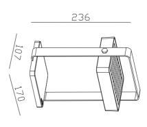
Voltage (V): 5 Volt IP degree: IP44 Class (Class 1, Class 2, Class 3): Class 3 (12V) Socket type: LED Module Switch placement: On the fixture
