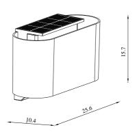
Voltage (V): 3,7 Volt IP degree: IP44 Class (Class 1, Class 2, Class 3): Class 3 (12V)
