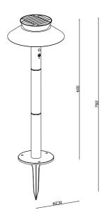
Voltage (V): 3,7 Volt IP degree: IP44 Class (Class 1, Class 2, Class 3): Class 3 (12V) Socket type: SolarLed
