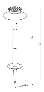
Voltage (V): 3,7 Volt IP degree: IP44 Class (Class 1, Class 2, Class 3): Class 3 (12V) Socket type: SolarLed
