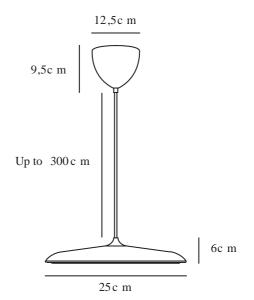
Voltage (V): 220-240 Volt IP degree: IP20 Class (Class 1, Class 2, Class 3): Class 2 (Double isolated) Socket type: LED Module
