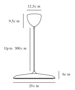
Tension (V): 220-240 Volt Protection IP: IP20 Classe (Classe 1, Classe 2, Classe 3): Classe 2 (Double isolation)
