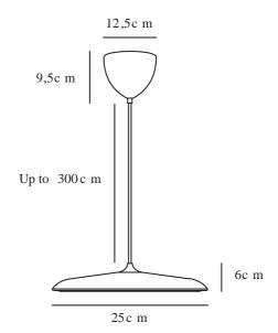
Voltage (V): 220-240 Volt IP degree: IP20 Class (Class 1, Class 2, Class 3): Class 2 (Double isolated) Socket type: LED Module Parallel connection: False
