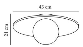
Voltage (V): 220-240 Volt IP degree: IP44 Maximum bulb wattage (W): 60W Class (Class 1, Class 2, Class 3): Class 2 (Double isolated) Socket type: E27 Parallel connection: False
